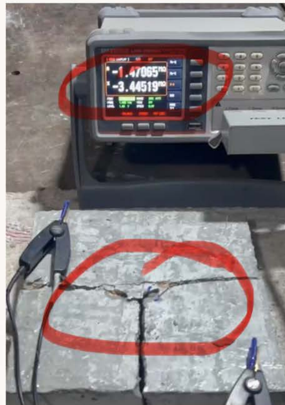
Resistance after severe cracking Externally visible
