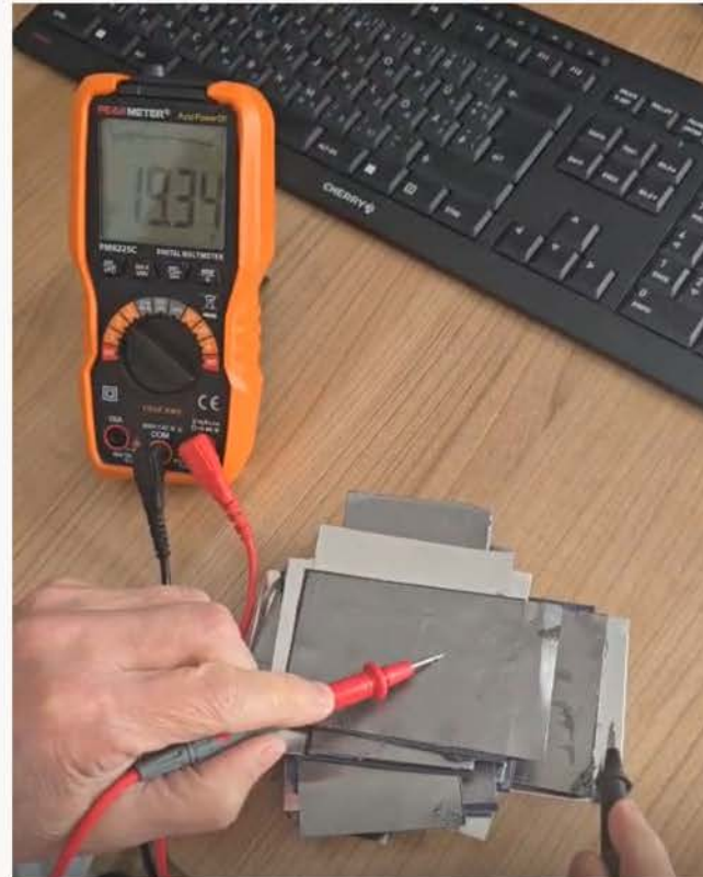
Measurement 10× storage plates – 19.34 V
